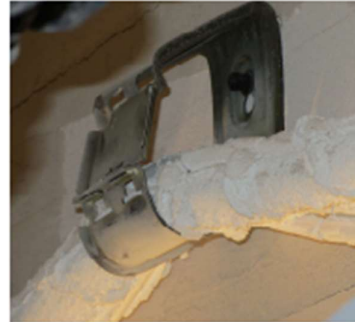
Fig 6: Deformation during wall mounting
